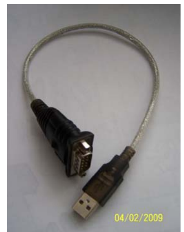
Figure 1. Adapter, serial (9-pin male) to USB. (See Section B.)
