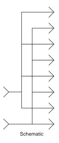
The NVT Model NV-EC4BNC is an adaptor used by NVT's IP transceivers to split a BNC signal four ways. It ships standard with the NV-EC1701-KIT3, NV-EC1701-KIT4, NV-EC1701-K3H, and NV-EC1701-K4H, but can be used with TBus products as well.
