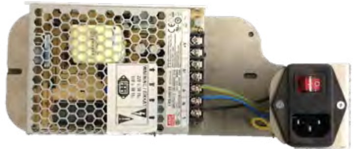
24 V DC POWER SUPPLY
