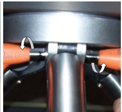
3. Tighten screws with 5 mm. keys
