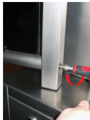
3. Tighten bottom fixing screw
