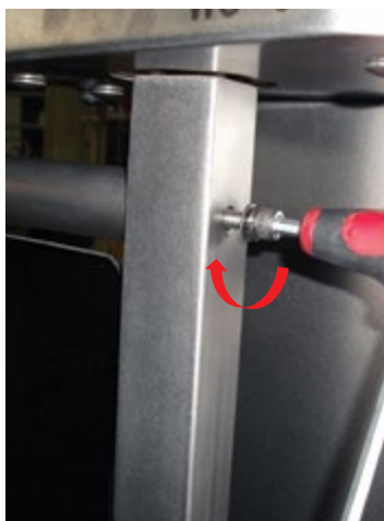
2. Tighten top fixing screw
