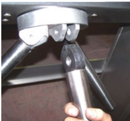
1. Seat the arm on the rotor
