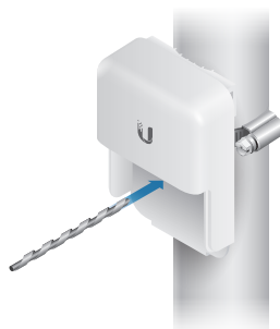
2. Drill a pilot hole into the pole.
