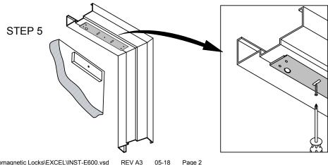
thickness only. From Armature side of door, drill 5/8" hole to insert reinforcement tube. Press in sexnut and reinforcement tube all the way and mount armature to door using hardware provided.
