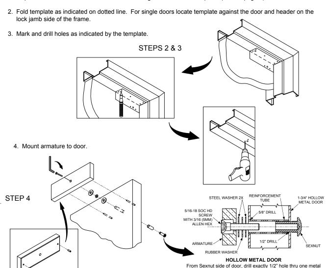
5. Install mounting plate to header with the interlock detail away from the door side of the stop. Loosely fasten screws through adjustment slot as shown. Assure that the mounting plate and armature line up properly, then tighten down ALL mounting screws.
