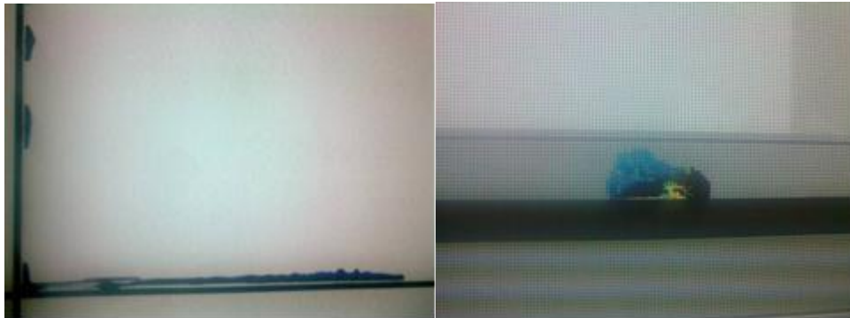
Figure 1-2 Liquid crystal leakage
