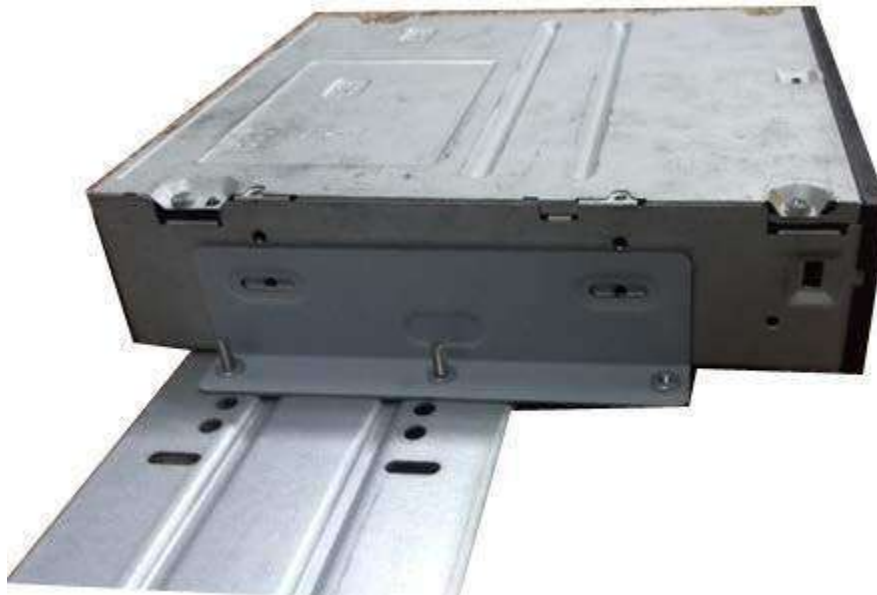
Figure 3-38 Install SATA burner
