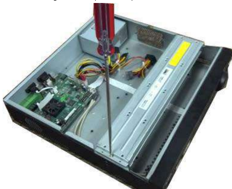
Figure 3-32 Open the top cover
