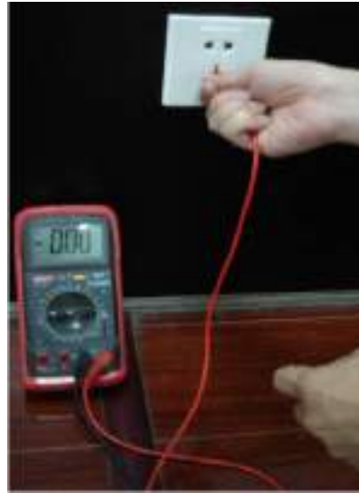
Appendix Figure 7-5 Check earth cable connection
