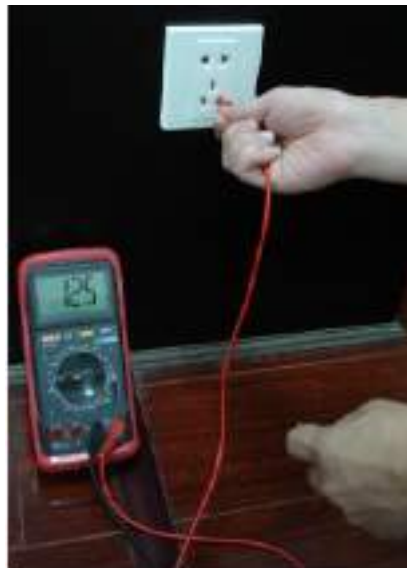
Appendix Figure 7-6 Check live cable connection
