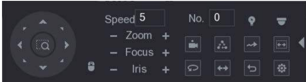
Figure 5-69 Expanded PTZ control panel
