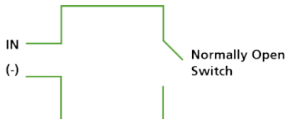
Figure 17: Normally Open Input Connection
