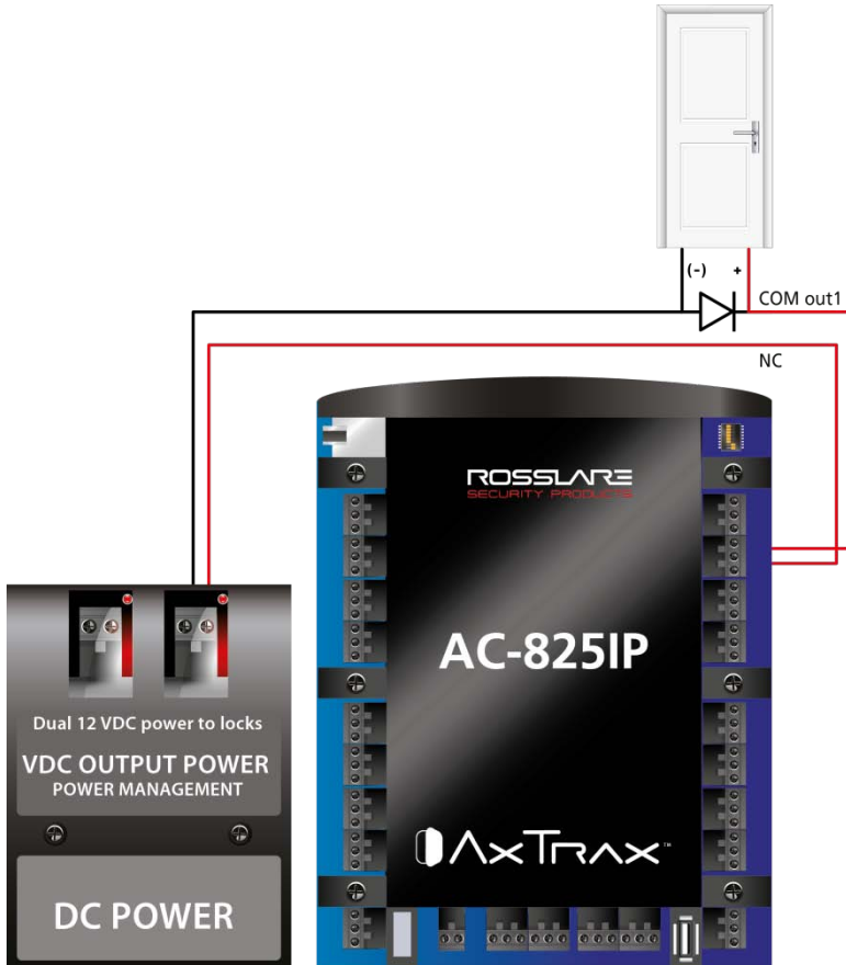
Figure 6: Door Lock – Failed Open
